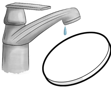
Clean the filters with water and let them dry. Filters should only be reinserted when completely dry.
